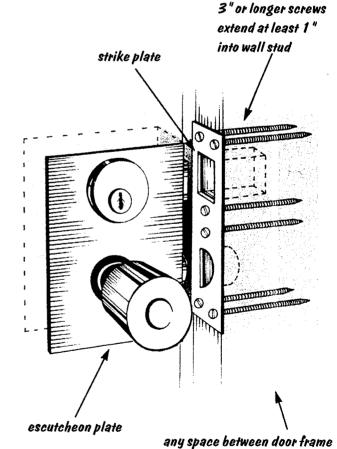
and wall stud should be filled with a hardwood insert
